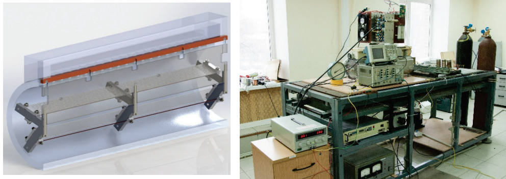
Fig. 1. a) Circulation chamber of electric discharge laser with four stage (cutaway). b) Experimental setup for the study of gas-discharge laser with EHD pumping system.
